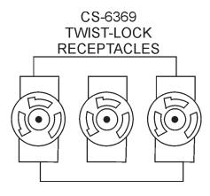
Figure 10. 240/139 VAC Twist-Lock Auxiliary Receptacles
